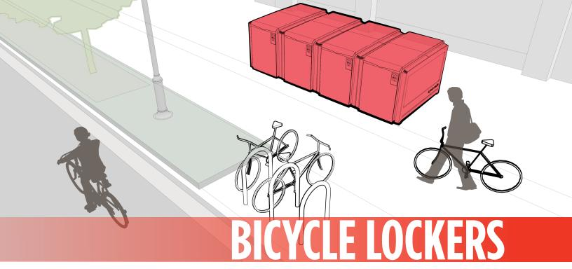
Bicycle lockers provide longer term bicycle parking than is typically provided by bicycle racks. Bike lockers securely protect a bicycle and its components as well as other related gear, including a helmet, bags, shoes, lights, and clothing from weather and theft.
